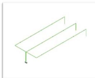
Remote test points were installed in each pipe run by extending the pipe down the far wall to an easy to access location, eliminating the need for expensive lifts during routine testing and maintenance.
